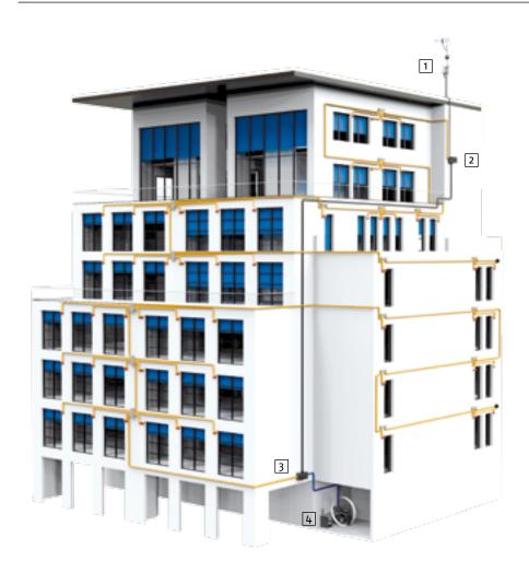
The animeo IP/RS485 Building Controllers and Sub Controllers are communicate bi-directionally with the motors.
