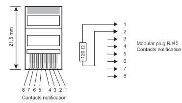
A RS485 component designed to terminate
