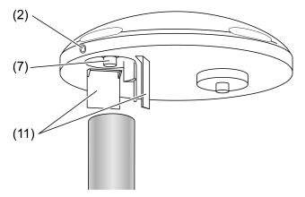
Figure 6: Mounting on freestanding mast without fastening arm
