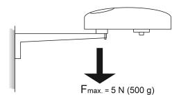
Figure 5: Maximum load on the fastening arm
