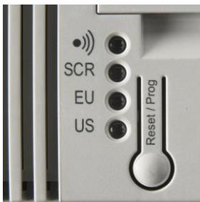
The "US"-LED blinks regularly when the mains (230 V) and the KNX bus voltage are connected actively on the device. The device is ready for operation when the "US" LED blinks.
