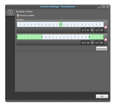
Picture 84: Function Settings - Security Timer - Solar shadings blocked during lunch and night.
