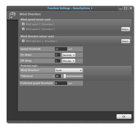
Picture 80: Function Settings – the Wind Direction function.
