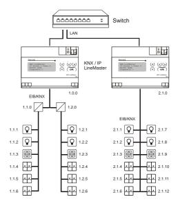
Fig. 3: KNX IP LineMaster as a backbone and line coupler
