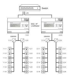
Fig. 2: KNX IP LineMaster as a backbone coupler
