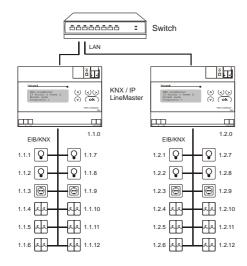
Fig. 1: KNX IP LineMaster as a line coupler
