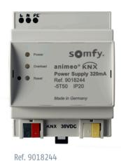
KNX Power Supply with integrated choke. Worldwide usable due to wide range input 100 – 240 VAC. LED indicator for Power, Overload and Reset. Push button for automatic reset on the KNX line. Additional auxiliary voltage output with 30 VDC. Nominal current on the short circuit protected outputs is 320 mA.
