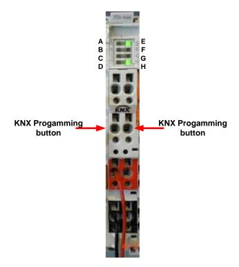
The red LED "B" on the KNX terminal blinks and shows that it is now in the active programming mode. Shortly afterwards, the green LED's "C", "H" and "E" will blink. The physical address of the KNX terminal has been programmed successfully when the green LED's "E" and "H" are continuously lit.
