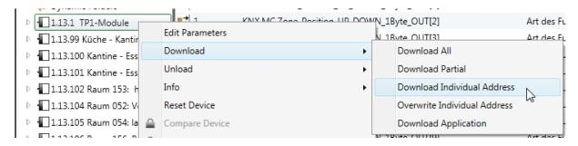
The yellow LED's "D" on the KNX terminal begin to blink. Make an electronic connection for a short moment between the KNX programming buttons (e.g. with a wire bridge).
