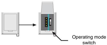
To activate the set IP address, a reset must be carried out on the animeo KNX Master Control. To do this, open the cover plate and press down the operation switch briefly using a screw driver. During pressing down, the LED's for "I/O" and "USR" shine red.
