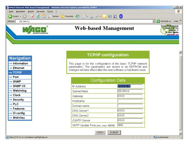
Now enter in the field "Configuration Data" under IP Address, the new desired IP address and likewise the subnet mask and confirm the entry with "Submit".
