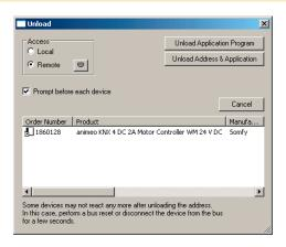
If the device with the ETS has already been programmed, a reset to delivery status is not possible over the Reset/Prog button. Over the function "Unload" in the ETS all settings of the device can be reset to delivery status. The Reset/Prog button can then be used again.
