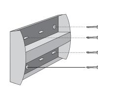
Mounting of the Motor Controller KNX 4 DC 2 A WM
