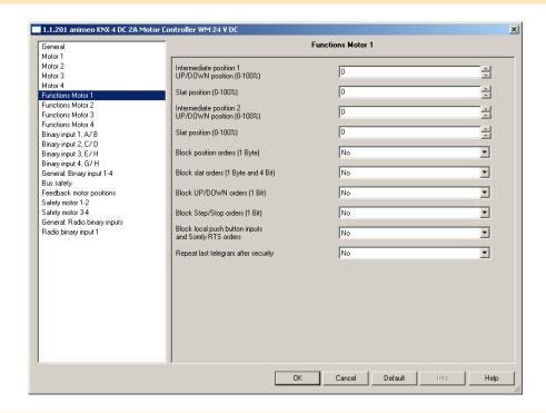
Four individual menu index cards (Functions Motor 1...4) become visible if on the menu index card "General" the basic adjustment of the motors is set to "Individual". Only one menu index card (Functions Motor 1-4) becomes visible, if on the menu index card "General" the basic adjustment of the motors is set to "Combined".
