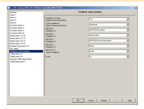
On this menu index card the parameters can be selected in order to announce the status positions of the individual blinds on the bus. The status positions generated thus are based on the configured running and tilting times of the menu index cards "Motor 1...4" or Motor 1-4".
