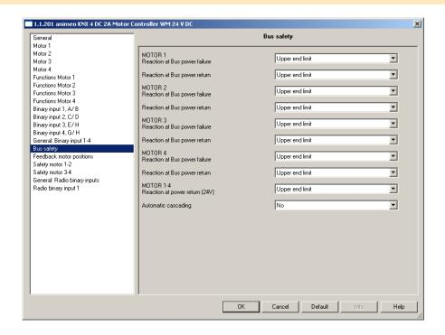
On this menu index card the reaction can be defined for bus power failure and bus power return of each individual motor output.
