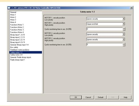
Two individual cards (Safety motor 1–2 / Safety motor 3–4) are visible when on the card "General" for the motor output configuration "Individual" is parametered. One card (Safety motor 1–4) is visible when on the card "General" for the motor output configuration "Combined" is parametered. The parameter for motor 1 is described as follows. The parameters for motors 2–4 are the same.
