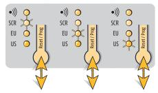
To switch between the different ergonomics press shortly the Reset/Prog button. Continue to do so until the desired LED is lighting.
