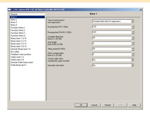
Four individual menu index cards (Motor 1...4) are visible when on the card "General" for the basic setting of the motor to "Individual" is parametered. An individual card (Motor 1-4) is visible when on the card "General" for the basic setting of the motor to "Combined" is parametered.
