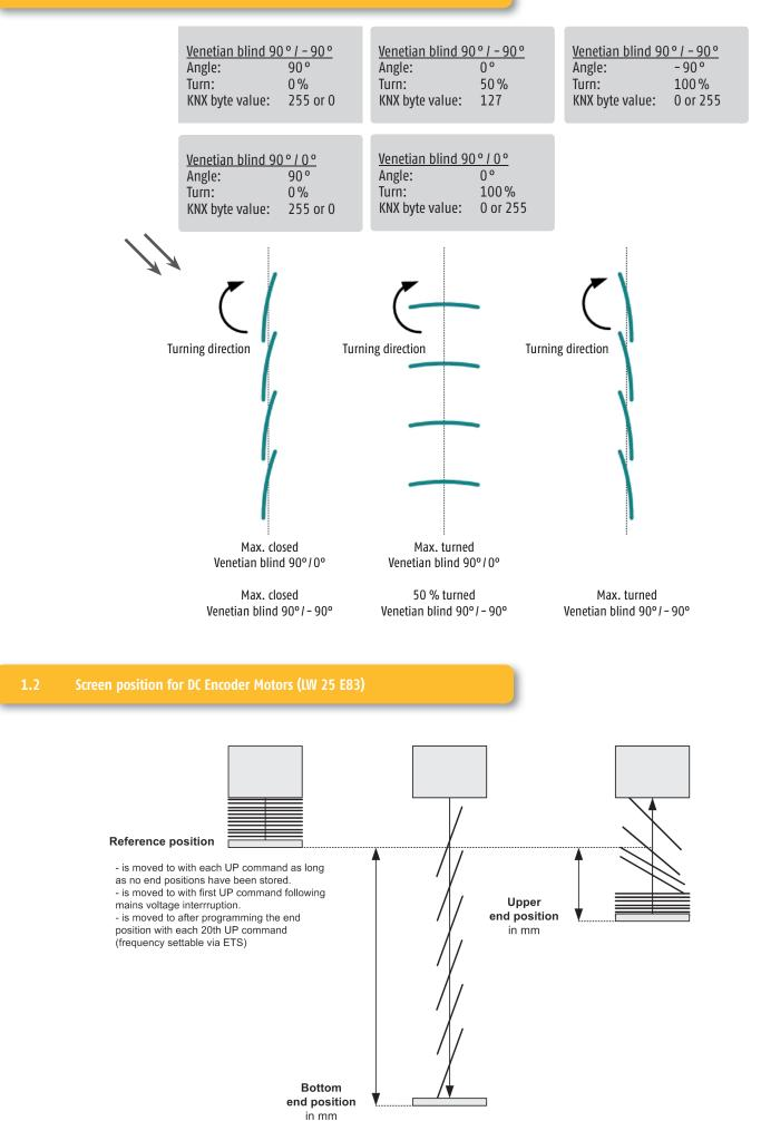
(lower edge of slats packet up to end position)
