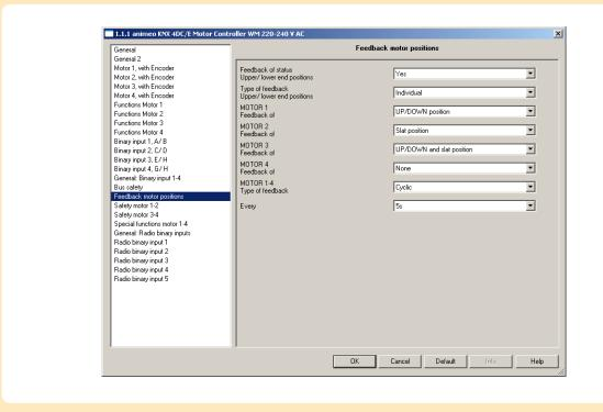
On this menu index card the parameters can be selected to announce the position status of the individual blinds on the bus. In addition, the generated status positions are based on the parametered running and tilting times of the menu index cards motor 1...4 or motor 1-4.
