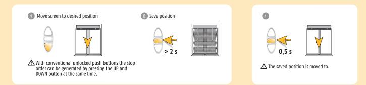
▲ When using DCE motors (LW25-E83) a complete UP command must be executed after learning-in the running and tilting times (lengths) so that the according blind can find its upper reference point.
